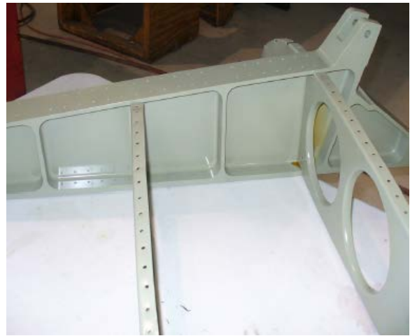
Pylon Fully Repaired
