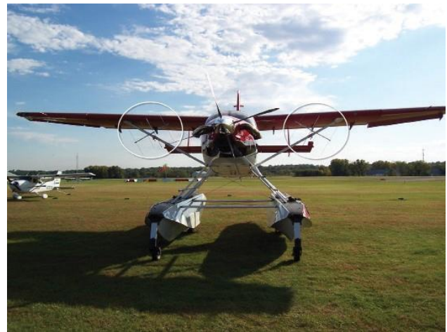
FIGURE A-1 YAGI ANTENNAS INSTALLED
