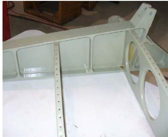
***Pylon Fully Repaired***
