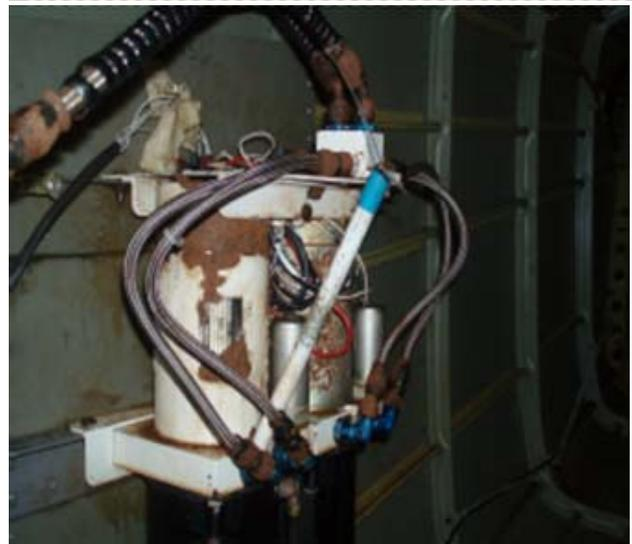
*Even without direct contact with saltwater, this hydraulic pump in the aircraft fuselage has severely corroded due to being in a saltwater environment without being kept clean.*
