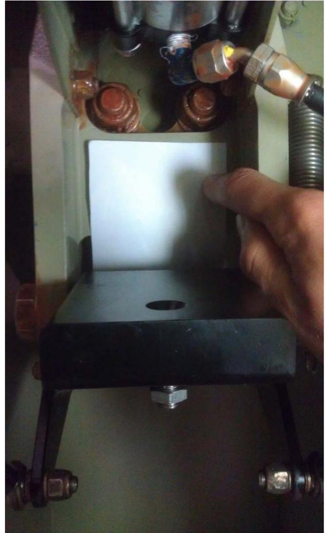
30. Loosen the (Fig 4-6, Item 1) jam nut on the Main Gear Down Stop Assembly, and screw in the NAS-428 adjustment bolt (Fig 4-6, Item 2). Verify the bolt does not touch the Top Arm when gear is in the down position. When the aircraft is off the jack stands and the weight of the aircraft fully on the
