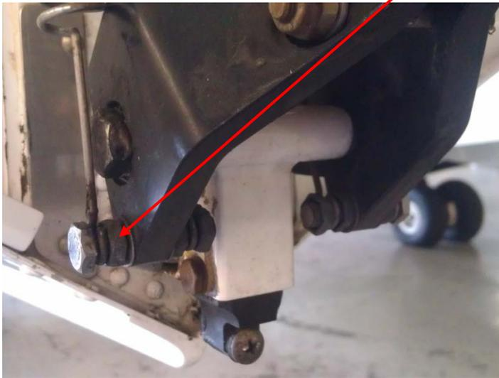
**Figure 2. 7000 water rudder springs lower bolt attachment.**
