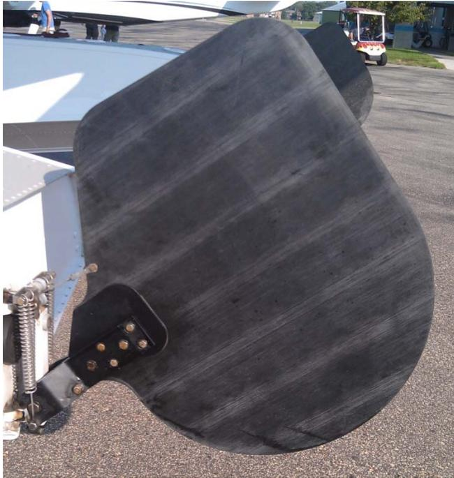
**Figure 6. Original 7000 float water rudder.**
