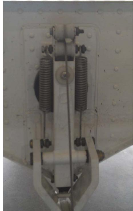
Figure 5. New spring attachment locations.
