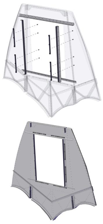
6. Backdrill through the 1003689 Horizontal Stiffeners in the 4 locations shown using a #30 drill bit
