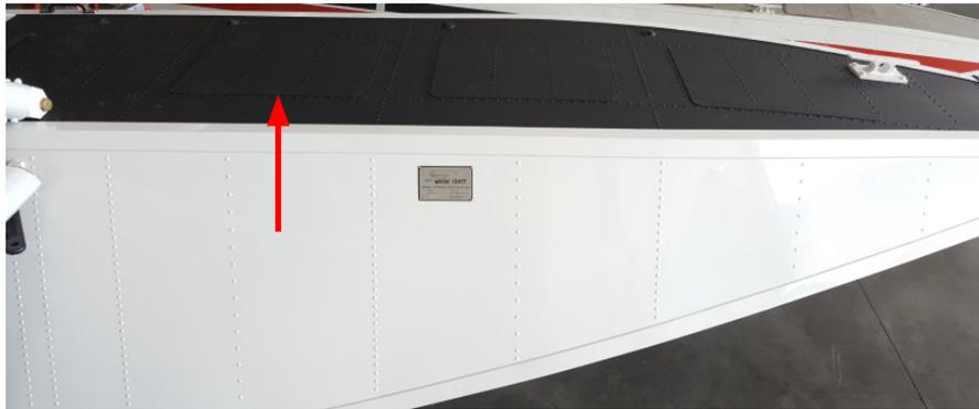
2. Inspect bulkhead 7 for cracking
