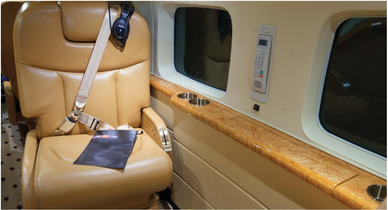
Custom side drink rails and retractable writing tables are constructed in composite material and covered in a light, wood grain, high gloss, veneer
