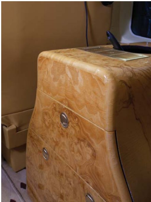
Custom side drink rails and retractable writing tables are constructed in composite material and covered in a light, wood grain, high gloss, veneer
