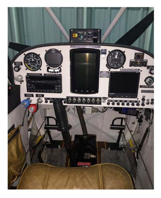
AVIONICS & Garmin 796 Weather and Music INSTRUMENTS Garmin GTX 327 Transponder Garmin SL 40 Com PM 3000 Intercom AK 451 ELT
