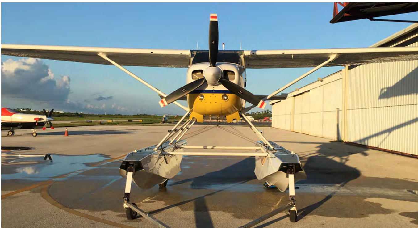
IO-550F Engine Upgrade and Wipline 3450 Floats
