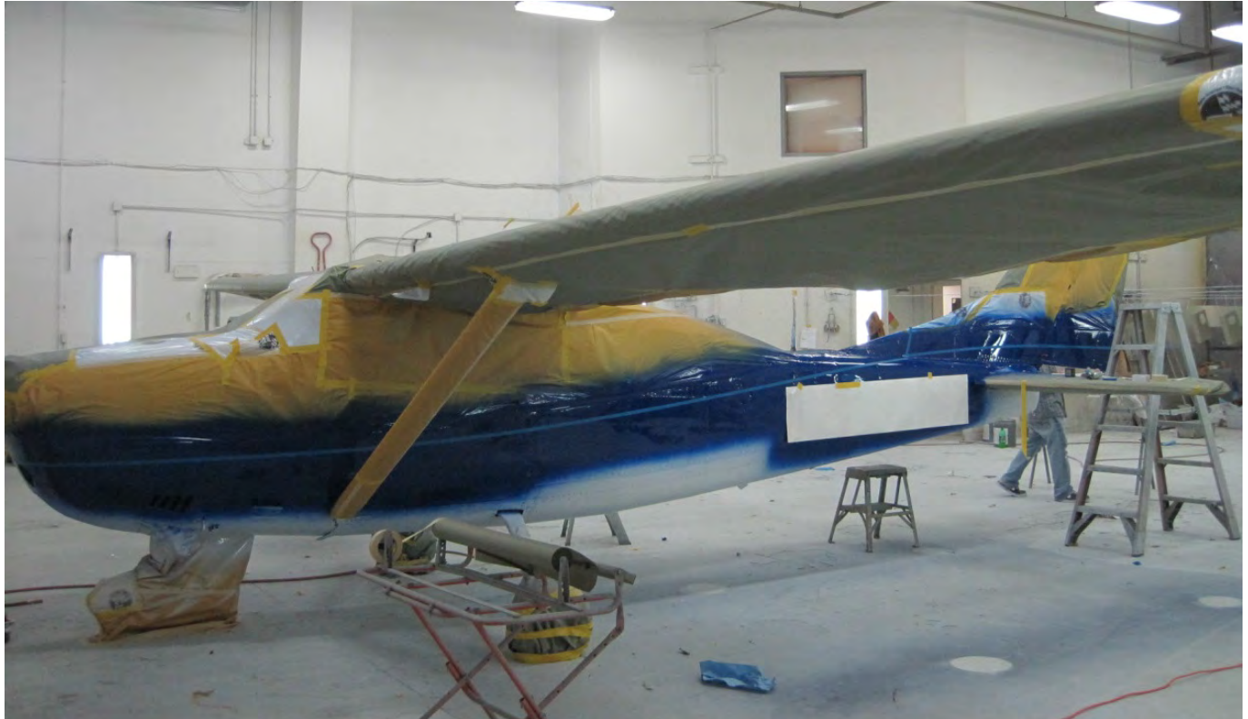
Paint Base Coat and Striping Being Completed
