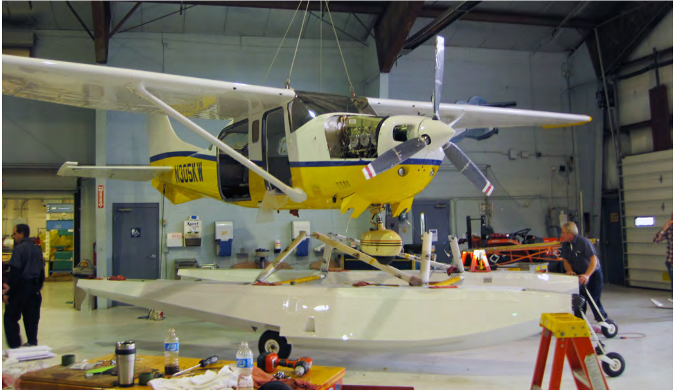
New Wipline 3450 Floats are Installed
