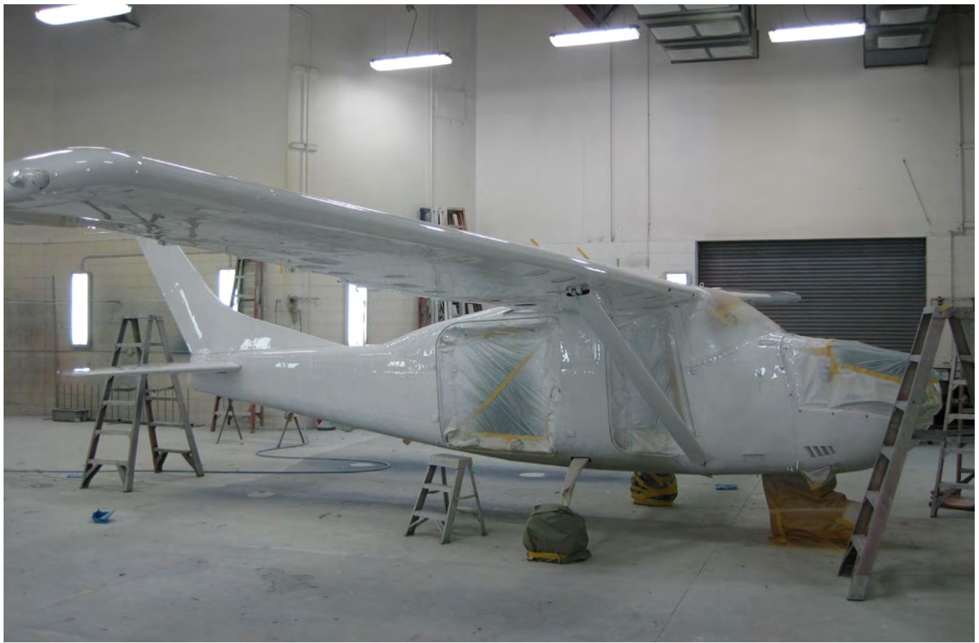
Paint Base Coat and Striping Being Completed
