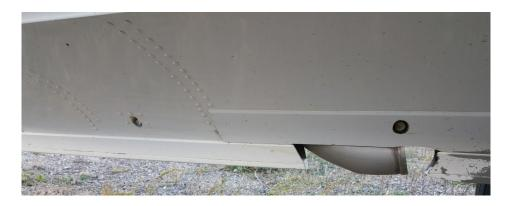
2. Gain access to the scoop tunnel assembly through the baggage compartment and by removing bulkhead 14 access panel
