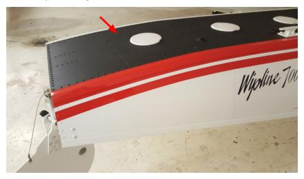
3. Drill out rivets that attach the existing gussets to the top deck (not shown), 1003229 water rudder pivot doubler, and 1005858 and 1005859 water rudder doubler angle supports as shown
