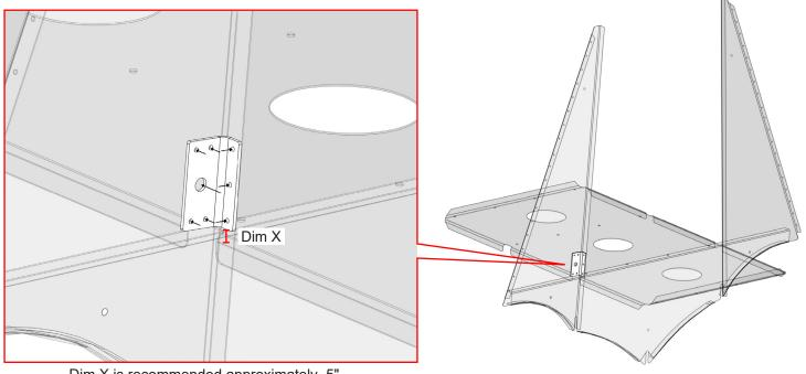
Dim X is recommended approximately .5" from the bottom of the doubler to the top of the baggage floor but may vary per installer discretion
