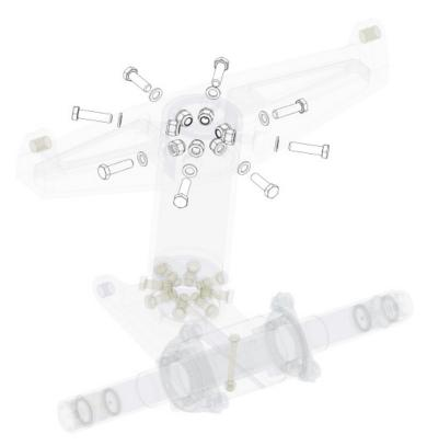
10. Remove the lower (8) AN bolts and associated (16) washers and (8) nuts.
