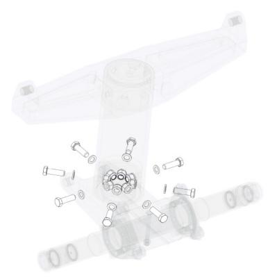
11. Separate the 8A04103-001 drag brace assembly, 8A04000-021 main gear axle assembly, and 8A04296-002 main gear drag brace tube
