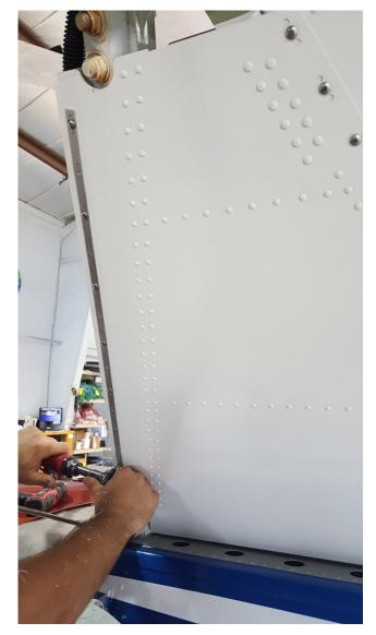
1008970 **NOTE:** Orient template so all holes align with existing hole locations
