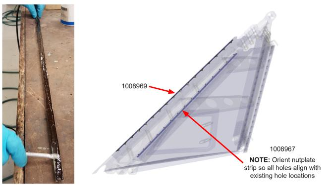
21. Temporarily install AN526C832R8 screws until sealer sets. Seal edges of nutplate strip assemblies with excess, previously applied sealer that seeped out from under the nutplate strip. Apply more if needed to cover all gaps between the nutplate strip and the main strut channel. Allow sealant to dry
