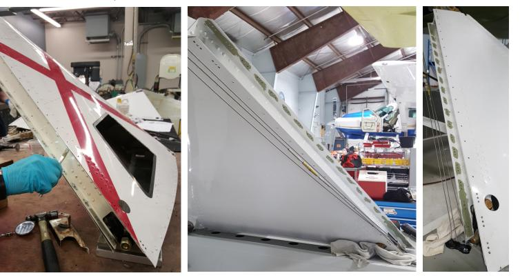
8. Apply a 1 inch piece of 9903-13-36 barrier tape to (4) MS21060L08 stainless steel nutplates and backdrill through tape in the locations shown
