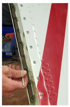
12. Apply a 1 inch piece of 9903-13-36 barrier tape to (5) MS21060L08 nutplates and backdrill through tape in the locations shown
