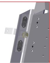
Note washer and nut behind Upper and Lower Pulley Brackets
