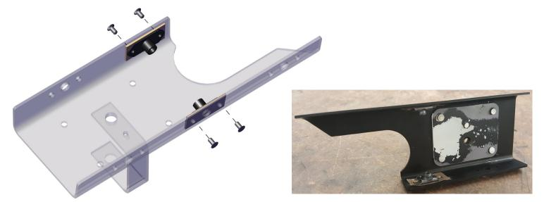
14. Position lower pulley bracket and nutplates inside of drag strut channel with clecos and install through drag strut channel with rivets MS20426AD3-4.5
