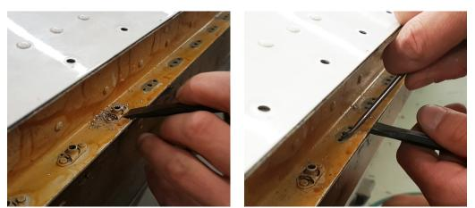
Pry off nutplate and remove rivet heads
