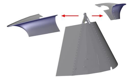
2. Remove leading edge and trailing edge pylon skins
