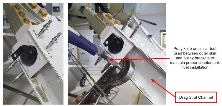
10. Apply PPG Aerospace PR-1422 B-2 sealer or equivalent to (2) 1008949 nutplate strip assemblies and install each one where shown
