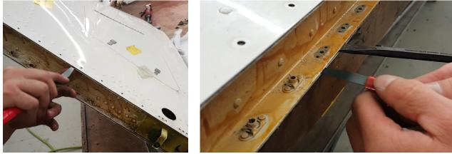
Remove aluminum chips between the skin and the channel
