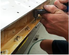
Grind or drill off rivet tails
