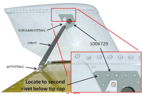
Figure 1: Support Strut Installation (Upper Right Finlet Shown – View Looking Inboard)
