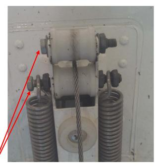
Figure 3. New bolts installed in upper and lower water retract cable pulleys.
