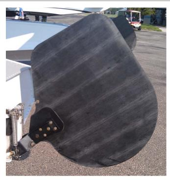
Figure 6. Original 7000 float water rudder.
