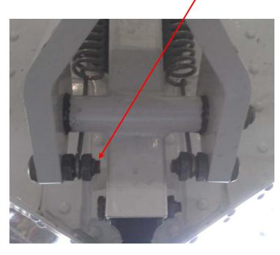
Figure 4. Lower spring attach bolts.
