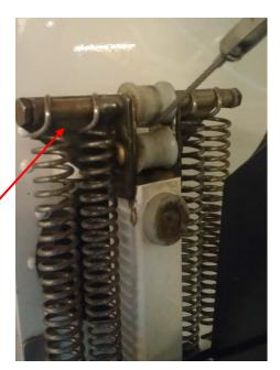
Figure 1. 7000 water rudder springs showing upper bracket.
