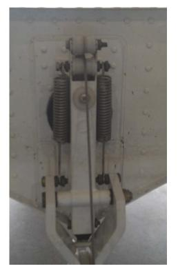
Figure 5. New spring attachment locations.
