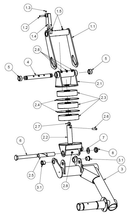
Diagram referenced from Wipaire parts manual. Bushing in question is item 3.1. Replace with flanged bushing (08FDU12 for 2100/2350; 10FDU10 for 3000/3450). Please refer to the service manual for your float model for information on removing the drag link and gear system.
