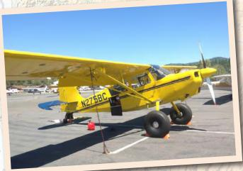
After being introduced to bush flying by Back-Country Aviation in Idaho, they introduced me to the American Champion Scout (8GCBC). It had the performance I was looking for; 70 gallons of fuel, 2100# gross (2600# restricted), composite propeller, and headroom! Alaskan Bushwheel 31" tires were installed and I received my tailwheel endorsement in my own Scout in Idaho.
