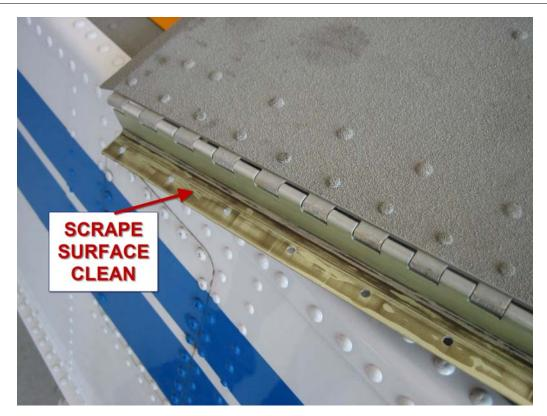
3. Cleco the Baggage Cover Lip and the Baggage Cover on so that the new Lip is flush with existing Lip. Ensure the holes line up.
