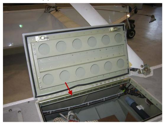
2. Scrape off old sealant from the hinge and Baggage Hatch edge.
