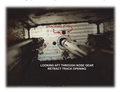
If evidence of cracking is found in Nose Box End Cap either by visual or dye penetrant inspection per figure 1, the following instructions will be accomplished to replace damaged Nose Box End Cap:
