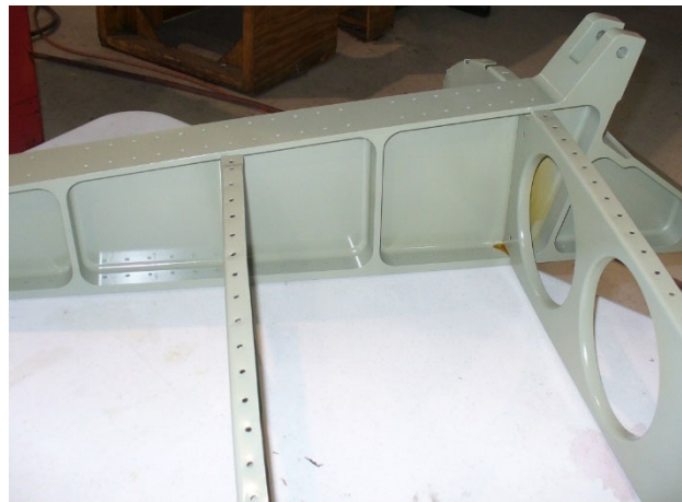
Pylon fully repaired
