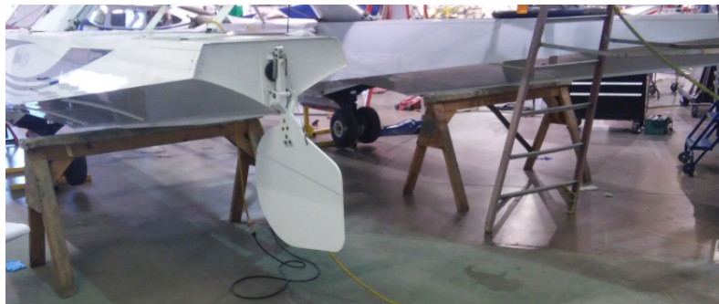
FIGURE 4-3 FLOAT SECURING LOCATIONS
