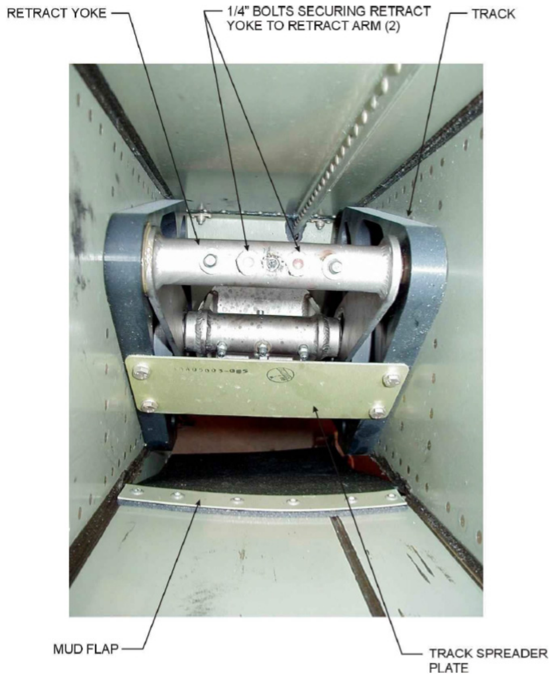
FIGURE 6-9 VIEW LOOKING DOWN THROUGH TOP ACCESS HOLE
