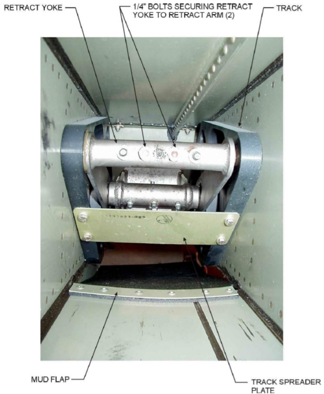
FIGURE 6-9 VIEW LOOKING DOWN THROUGH TOP ACCESS HOLE
