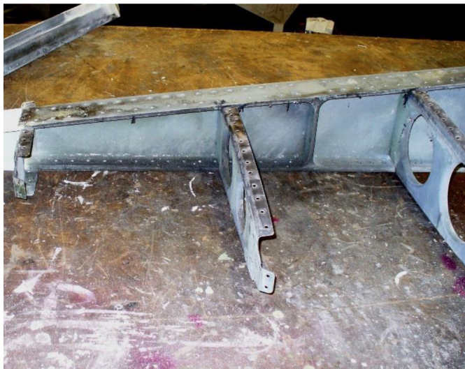
Pylon before repair
