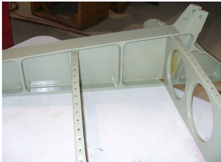
Pylon fully repaired
