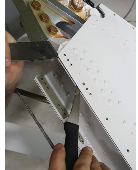
Remove rivet heads and aluminum chips between the skin and the channel
