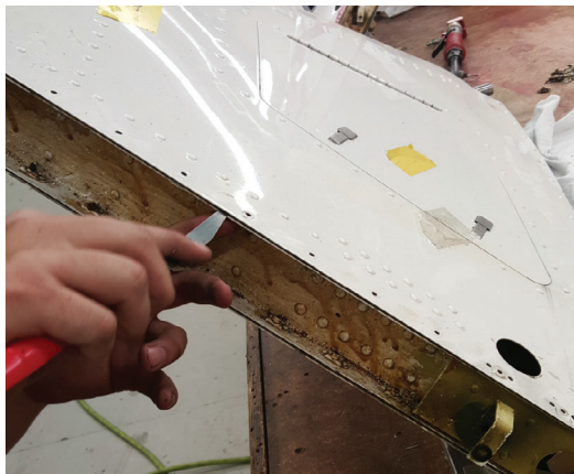
Remove aluminum chips between the skin and the channel
