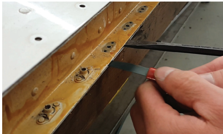
Remove aluminum chips between the skin and the channel
