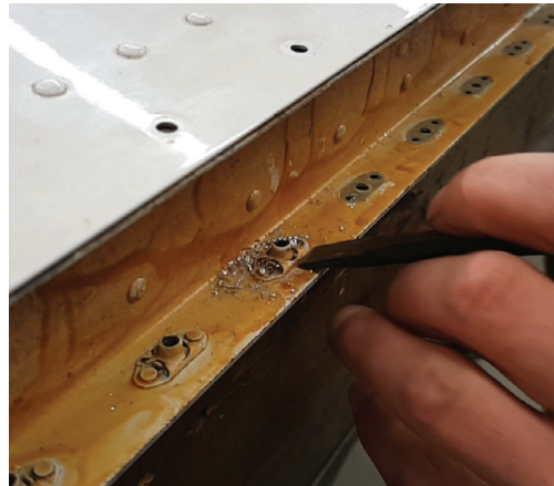
Pry off nutplate and remove rivet heads
