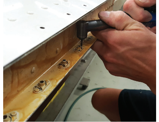
Grind or drill off rivet tails
