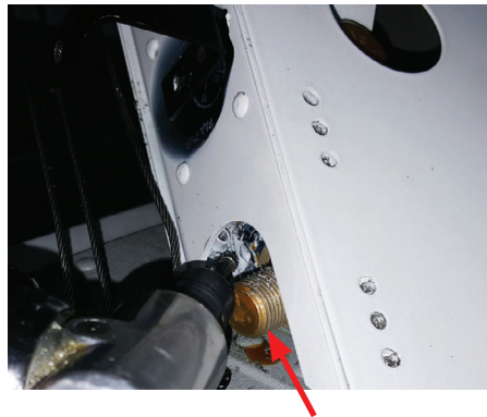
Remove nut to gain access to rivet locations
