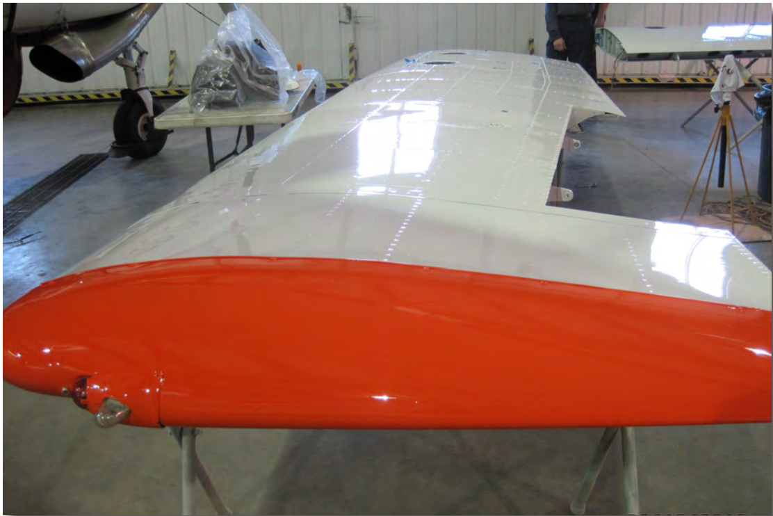
"Wip" Tip Wing Extensions Installed
