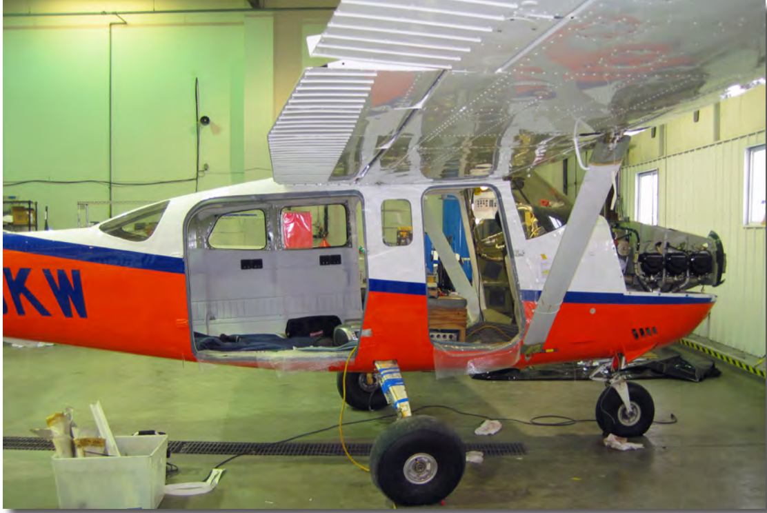
Wipaire's Co-Pilot Door STC Install
