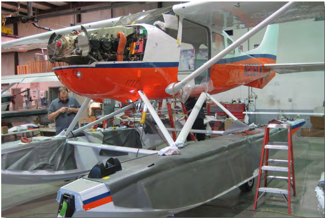
New Wipline 3450 Amphibs Installed
