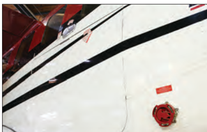
Single Point Fueling System
