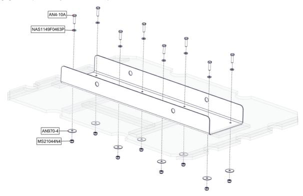
4. If previously removed, reinstall baggage floor panel with attached 1009883 anchor channel and verify the baggage floor panel is securely attached to the forward and aft bulkheads
