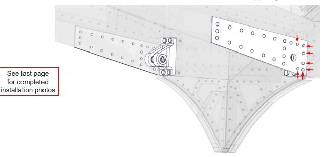
NOTE: During reassembly, replace any hardware that shows signs of corrosion.
