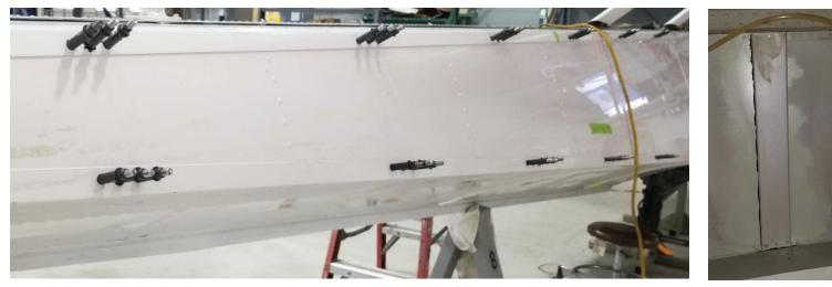
6. Rivet stiffeners to side skins at the top and bottom as shown below.
