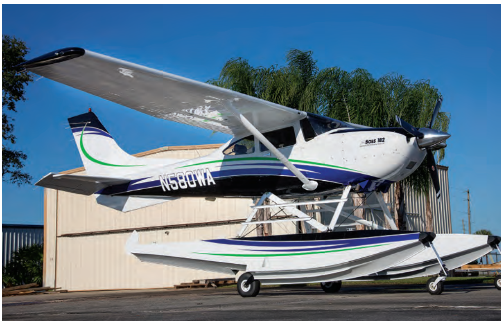
The Lycoming IO-580 boosts the Boss 182's climb rate to over 1,000 fpm on Wipline 3000 amphib floats.
