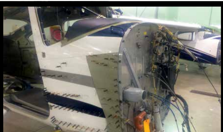
Extensive airframe modifications include fuselage skin doublers in the area where forward float struts attach.
