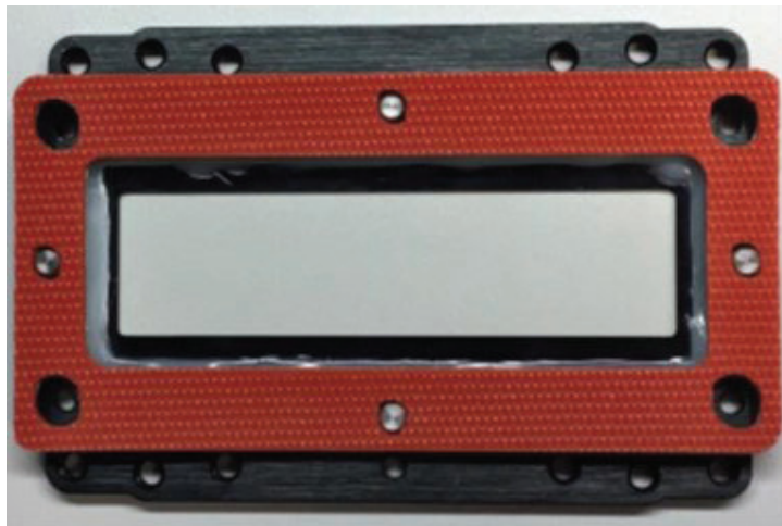
Figure 3 – Faceplate with Internal Gasket
