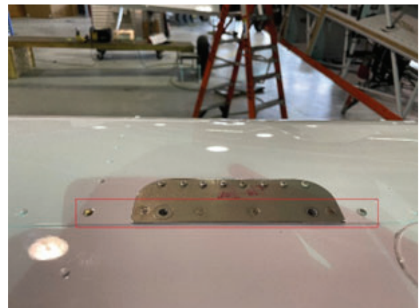
Figure 2 Stabilizer forward spar strap locations (LH stabilizer shown, RH is primary concern)
