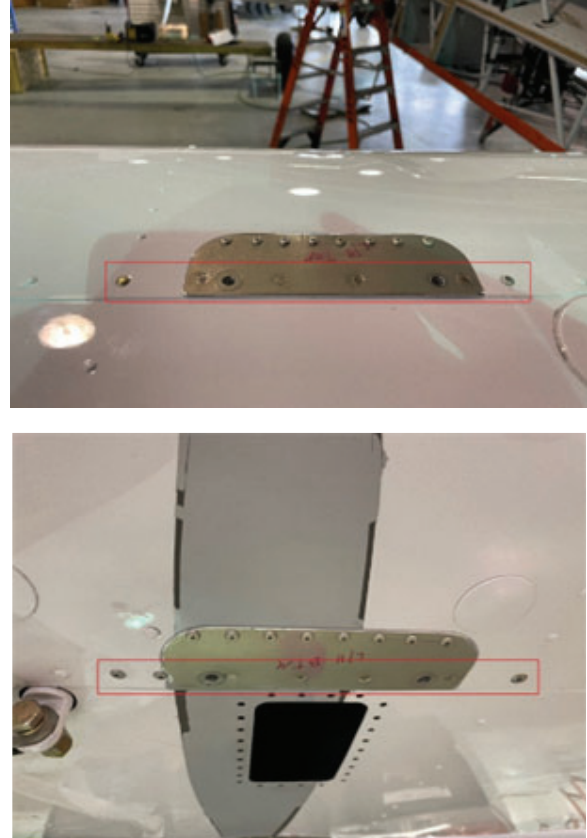
Stabilizer forward spar strap locations (LH stabilizer shown)
