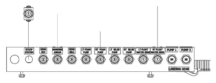
5. Install the 2 amp circuit breaker, part number 7277-2-2, by performing the previous steps in reverse.
